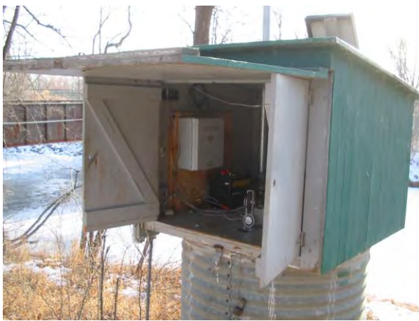
Automated river gage located on Clearwater River at Plummer
