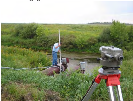
Surveying water lift from river to pump
