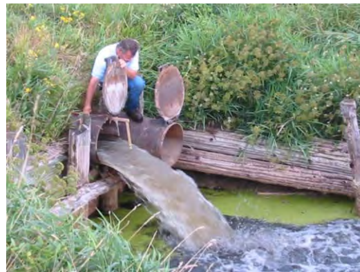
Measuring flow using manual method
