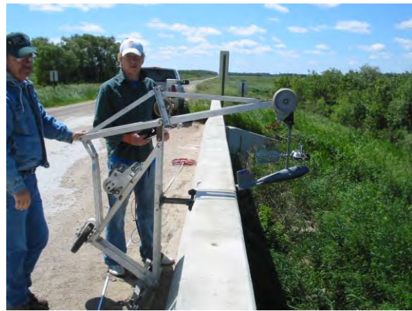
Measuring flow with bridge crane
